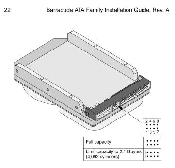
Figure 5. Alternate Capacity Jumper
