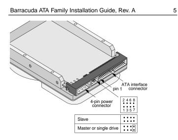
Figure 1. Master and slave jumper settings
