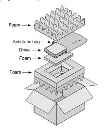
Figure 6. Seagate drive and approved packing materials
